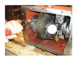
27. Mount indicator base on the power frame (1) with the indicator tip on a machined shoulder surface of the crankshaft (2) (do not measure from a cast surface) and the axis of the indicator parallel to the crankshaft (2).
