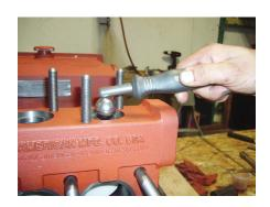
7. To remove the ball valve seat use knock out tool PPAM A000233000. Use tool PPAM A000399000 for disc valve
