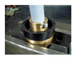
9. Inspect all parts for damage or unusual wear. Ensure that the interior surface of the cylinder (39) is smooth and free of cracks or grooves. New piston cups (40) will fail prematurely if installed in liners with damaged bores. American Mfg Company strongly recommends that all three piston cups be replaced, not just those that show signs of leakage, whenever this type of service is performed. This will maximize operational time between service intervals.
