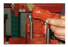
5. The cylinder covers (54) allows access for inlet valve removal. Remove the cylinder covers as described in section (9.1), steps 1 through 9.
