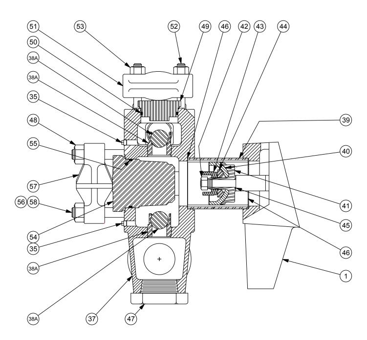
Figure 3A Pump AL1122BCD: Fluid End Components
