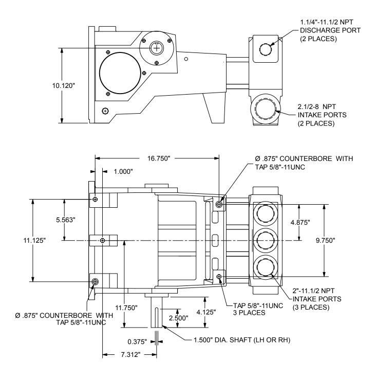
Figure 7: Pump Mount Bolt Pattern
