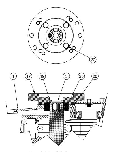
Figure 4: Spline Shaft Components
