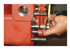
6. Following the hex piston nut (42) removal, use the American Mfg Company piston tool (PPFMC A5049) to pull the piston assembly from the cylinder (39). Insert the American Mfg Company piston tool inside the cylinder until flush with the face of the slotted piston retainer nut (43). Twist the tool to engage and lock the tabs of the tool inside the mating slots in the retainer nut.
