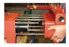
4. Rock the fluid cylinder (fluid chamber) to loosen from the cylinders (liners) (39), and then pull free of the fluid end studs. If the pistons have already been removed, take care to ensure that the cylinders (liners) do not fall off of the front of the power end and become damaged.
