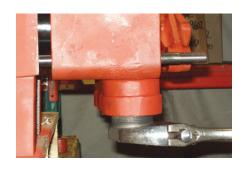
4. Remove the six valve cover nuts (53) holding the valve cover clamps (51) and then remove the three valve covers (49) from the fluid cylinder.
