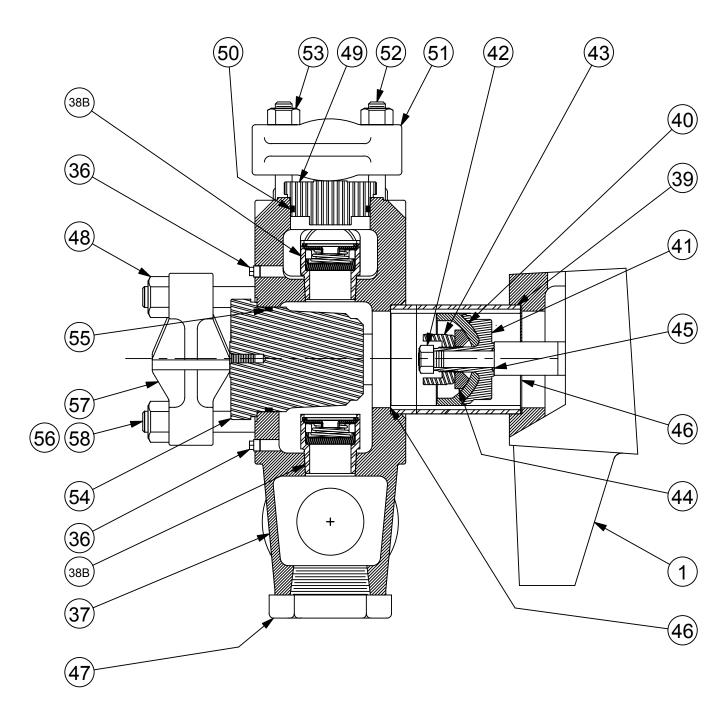
Figure 3B Pump AL1122D: Fluid End Components
