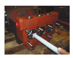
7. Pull the piston assembly free of the pump using a combination pulling and twisting motion.
