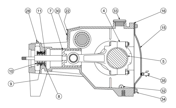
Figure 2B: Power End Components
