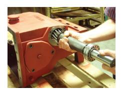
7. The pinion shaft (3) with bearings may then be removed from the drive side by using a brass rod (or other soft material) and mallet to drive the shaft out.
