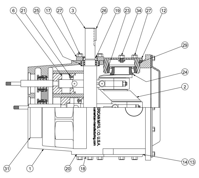
Figure 2A: Power End Components
